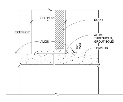
8 Transition Concrete to Concrete S8 3" = 1'-0"
