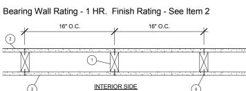
1. Wood Studs - Nom 2 by 4 in. spaced 16 in. OC, effectively cross braced at mid-height and fire stopped at top and bottom.
