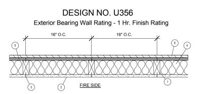
Wood Studs - Nom 2 by 4 in. spaced 16 in. OC with two 2 by 4 in. top and one 2 by 4 in. bottom plates. Studs laterally-braced by wood structural panel sheathing (Item 5).
