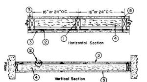
Wood Studs -- Nom 2 by 4 in., spaced 16 or 24. OC. Effectively cross braced. **Resilient Channel** -- 25 MSG galv steel. Resilient channels spaced vertically 24 in. OC, flange portion screw attached to one side of studs with 1-1/4 in. long diamond shaped point, double lead Phillips head steel screws.
