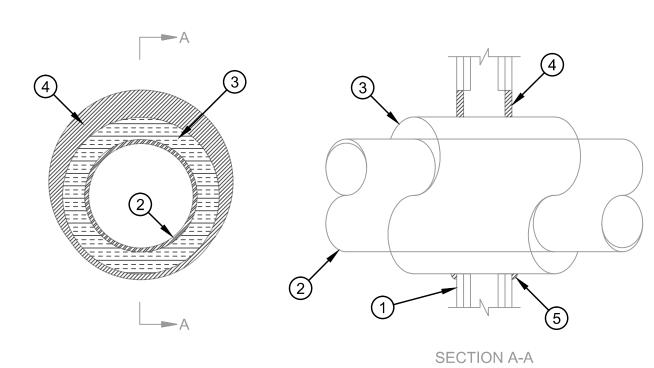
1. Wall Assembly— The 1 or 2 hr fire-rated gypsum board/stud wall assembly shall be constructed of the materials and in the manner specified in the individual U300 or U400 Series Wall and Partition Designs in the UL Fire Resistance Directory and shall include the following construction features:
