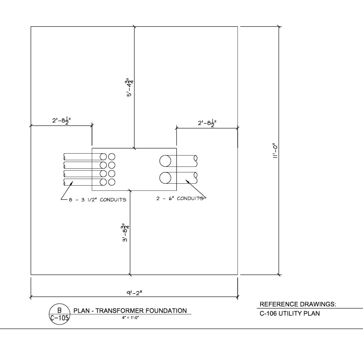
9. <u>SLAB FOUNDATION SUPPORT</u> SEE POWER CO. ELECTRIC STANDARDS <u>8.10</u> FOR ADDITIONAL INFORMATION. A. THE FOUNDATION DESIGN MUST HAVE THE SIGNED APPROVAL OF THE POWER CO. REPRESENTATIVE. B. ONE COPY OF THE PLAN FOR THE TRANSFORMER SLAB INSTALLATION AND FOUNDATION DESIGN MUST BE FILED WITH POWER CO. / ENGINEER OR REPRESENTATIVE PRIOR TO CONSTRUCTION OF SLAB. PIPE SLEEVES INSTALLED IN THE TRANSFORMER SLAB, THE 4 INCH PIPE SHALL BE REMOVABLE.
