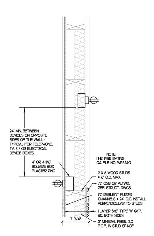
NOTE: LAYOUT OF BOXES ON OPPOSITE SIDES OF WALLS MUST BE APPROVED BY THE LOCAL FIRE MARSHALL PRIOR TO CONSTRUCTION
