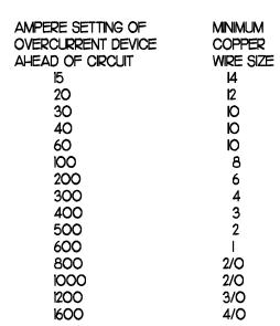
5. GROUND SERVICE TO WATER PIPE, GROUND ROD, AND CONCRETE ENCASED ELECTRODE WITH ARTICLE 250 OF THE N.E.C.
