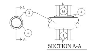
1. FLOOR OR WALL ASSEMBLY- MIN.2-1/2 in. THICK REINFORCED LIGHTWEIGHT OR NORMAL WEIGHT (100-150 PCF) CONCRETE. WALL MAY ALSO BE CONSTRUCTED OF ANY UL CLASSIFIED CONCRETE BLOCK\*. MAX. DIAM. OF OPENING IS 6 in. .
