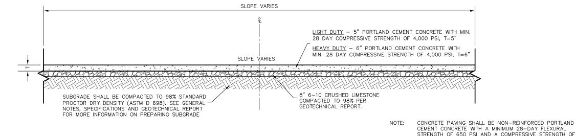
4,000 PSI. JOINT SPACING, JOINT CONFIGURATION, MIX DESIGN, MIX PLACEMENT, AND CURING SHOULD CONFORM TO THE RECOMMENDATIONS OF THE AMERICAN CONCRETE INSTITUTE (ACI) AND THE PORTLAND CEMENT ASSOCIATION (PCA). TYPICAL SECTION OF RIGID PAVEMENT STRUCTURE
