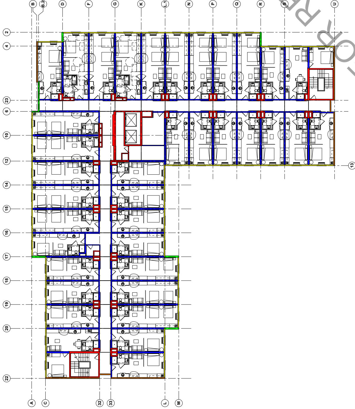
① LEVEL-4 BUILDING FIRE SEPARATION PLAN 1/8" = 1'-0"
