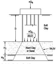
Equivalent Footing at Depth D Settlement of Pile Group - Compression of Layers H1 and H2 Under Pressure Distribution Shown.
